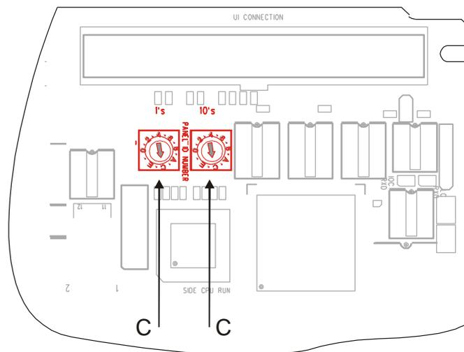
Rotary switches set to CC on mc2 board
