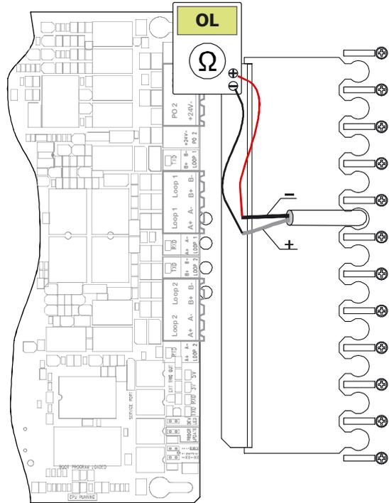
3. Short-circuit the monitored output line cable wires at the control panel during measuring.
