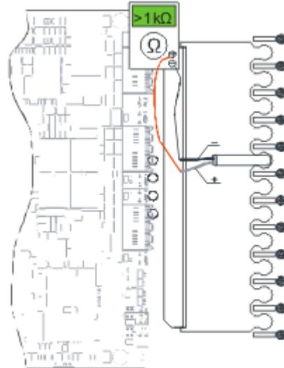
2. Measure the loop cable + wire resistance from the output and return ends. Also measure the - wire. The loop resistance of the + and - wires added together can be max. 60 Ω on SLC - loop and 60 Ω on ALC - loop.
